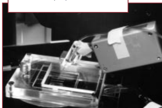
MIF device on a microscope stage with an electrophysiological micropipette lowered into the recording chamber.
